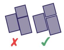
Never butt joint paving when laying you should always use an appropriate joint for your chosen product. Global Stone products should be laid with a minimum 8-10mm joint.
