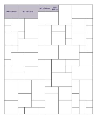
All dimensions shown are nominal, pattern includes 10mm joints approximately. Always mix slabs (whilst laying) when using multiple packs.
