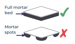
Always lay paving on a full bed of mortar and never use the spot bed method – see our step by step laying guides for more advice on this.
